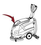
Adjust the slope of the handle by pulling the handle release lever.
